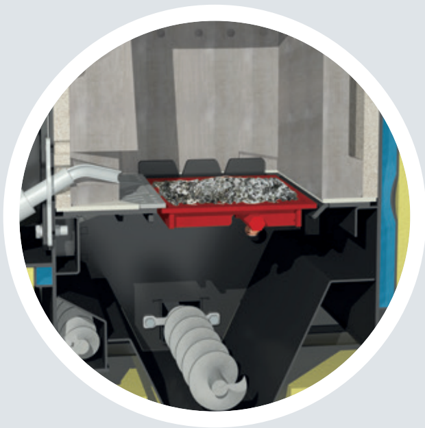
Two-part combustion grate consisting of a fixed insertion zone and automatic tipping grate guarantee energy-saving operation and lowest emissions.
