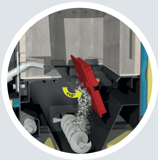
Due to the 110° inclination, the ash is completely emptied from the tipping grate and discharged into the large-volume mobile ash container by means of the ash screw.
