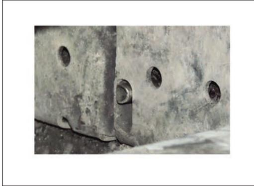
**NOTICE!** The igniter tube must protrude approx. 0.5 to 1 cm over the combustion chamber guard.
